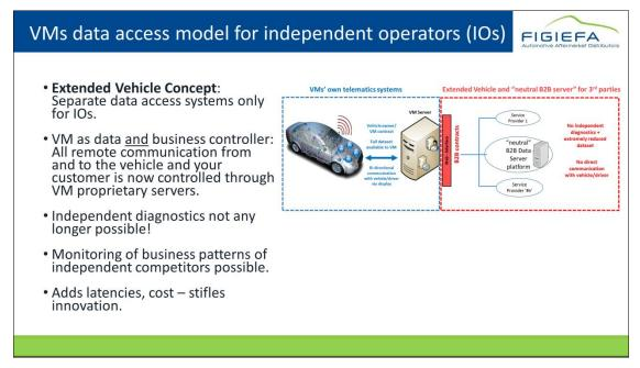
Note: In the latest version of this ExVe concept, a so-called "neutral server" is linked behind the ExVe backend server (the so-called "**NEVADA**"<sup>9</sup> concept). It is a B2B data brokering platform of third party service providers which is hooked behind the ExVe system. As such, it does not remedy any of the systemic failures created by Extended Vehicle, but instead, adds further costs, contractual conditions and latencies.
