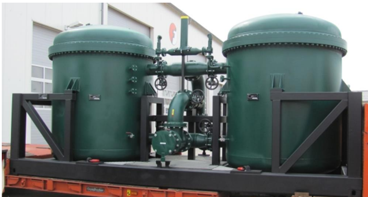
Figure 14: Example Fangmann Industrie – separator skid with two adsorbers (DN 250; DP64)
