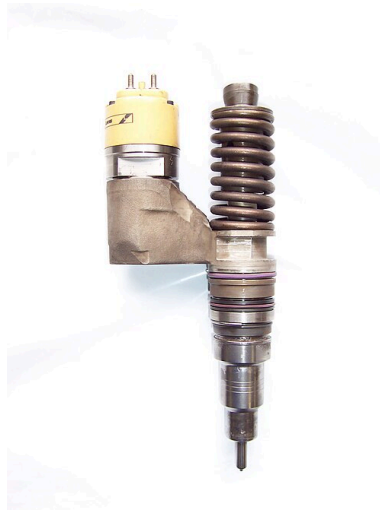
Early Lucas electronic diesel unit injector
