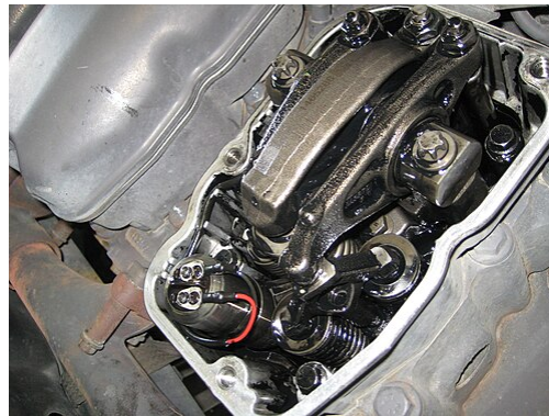
Bosch UI on a Scania R164 V8 engine
