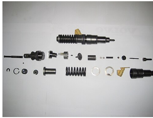
Delphi E1 unit injector parts
